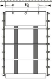
4. Insert the lift into the installation board, and use four pcs bolts (M6\*12) to fix them.
