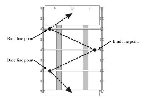
(Before binding the wires, please have the lift down to the projector working position)
