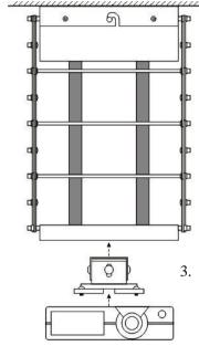
Install the universal head and claws to fix the projector.
